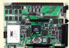
HERCULES II EBX SBC CPU, I/O, DAQ and DC power supply on one board
